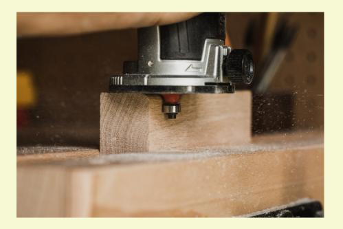
A router is a power tool with a flat base and a rotating blade extending past the base. The spindle may be driven by an electric motor or by a pneumatic motor. It routs (hollows out) an area in hard material, such as wood or plastic.
